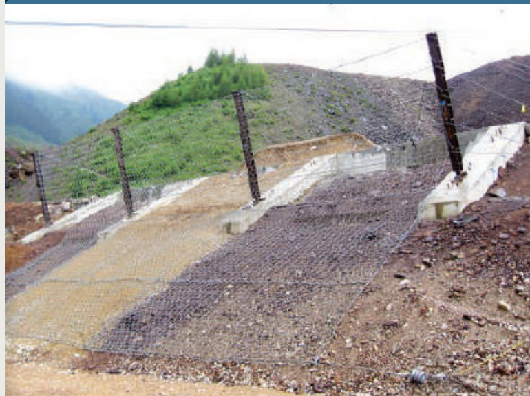
Before photo of a 3000 kJ hybrid test. The system consists of 5 m high posts with 12 m of Omega-Net.
