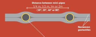
Perforated mini-pipes diameter 16 mm, 20 mm or 25 mm
